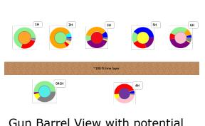
Gun Barrel View with potential lime frac barrier
